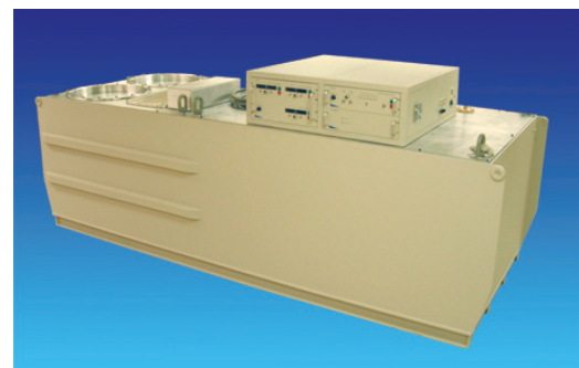
DTI's hybrid modulator. The capacitors, 80 kV solid-state switch, and a 6.33:1 pulse transformer are insulated by transformer oil and reside in two isolated sections of a single large tank. System controls are in the small enclosure on top of the tank.
