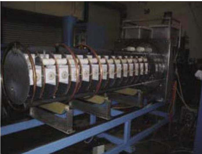
Marx generator capacitor chain
